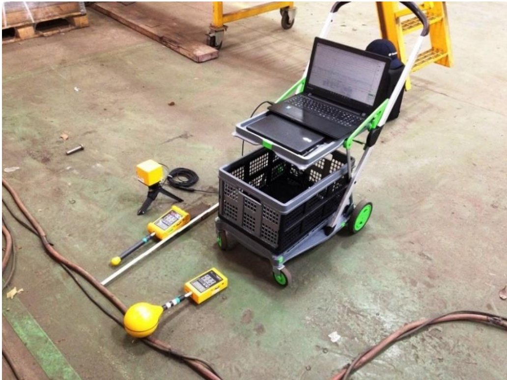
Figure 3 Measuring time-varying, low frequency magnetic fields using the Narda EHP-50 device, Narda ELT-400 probes and associated equipment.
