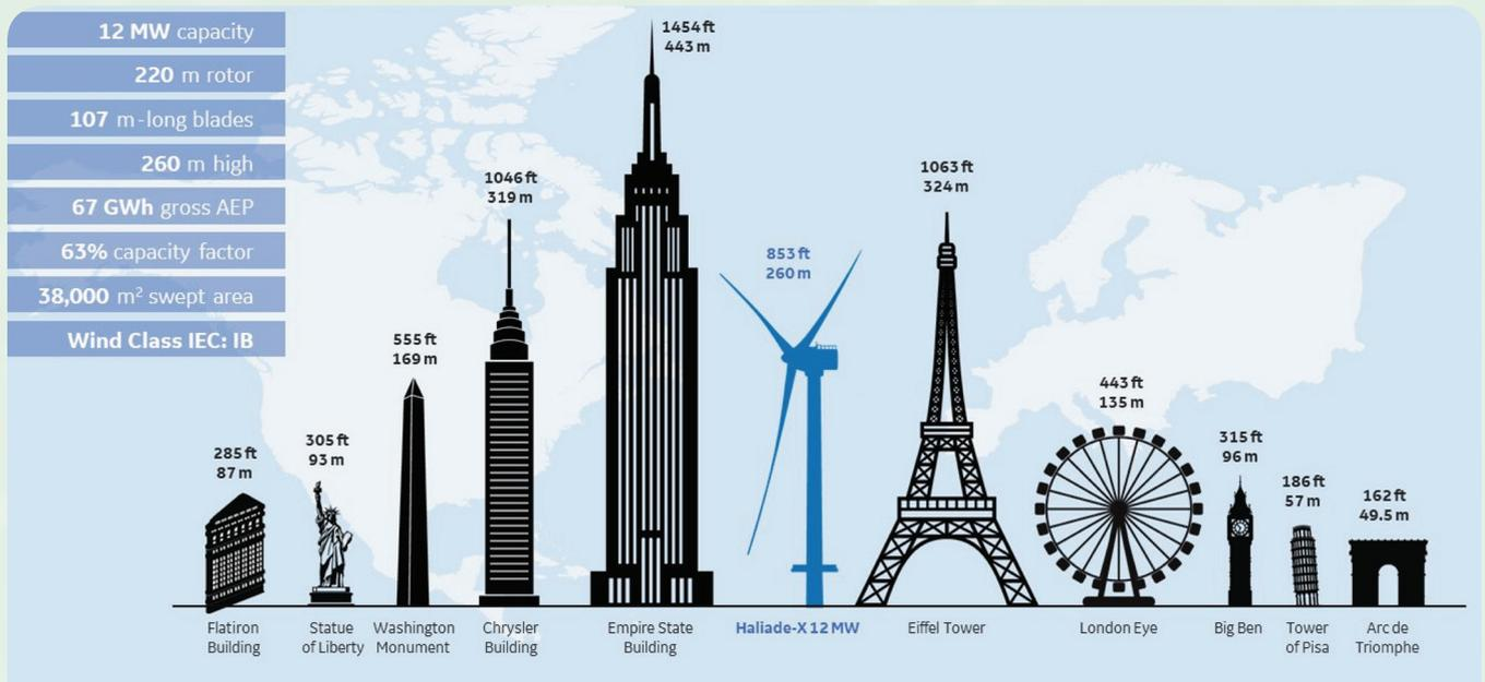
Figure 1. Comparison of the GE Haliade-X 12 MW wind turbine with other well-known structures
