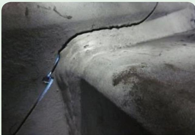
Figure 20. Cracking in a nacelle bedplate. The full length of this crack is over a metre
