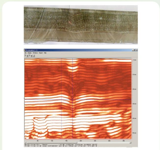
Figure 23. Example of a wrinkle in a blade structure and an ultrasonic B-scan cross-section
