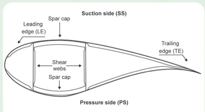
Figure 14. Cross-section of a wind turbine blade showing components referred to in the text
