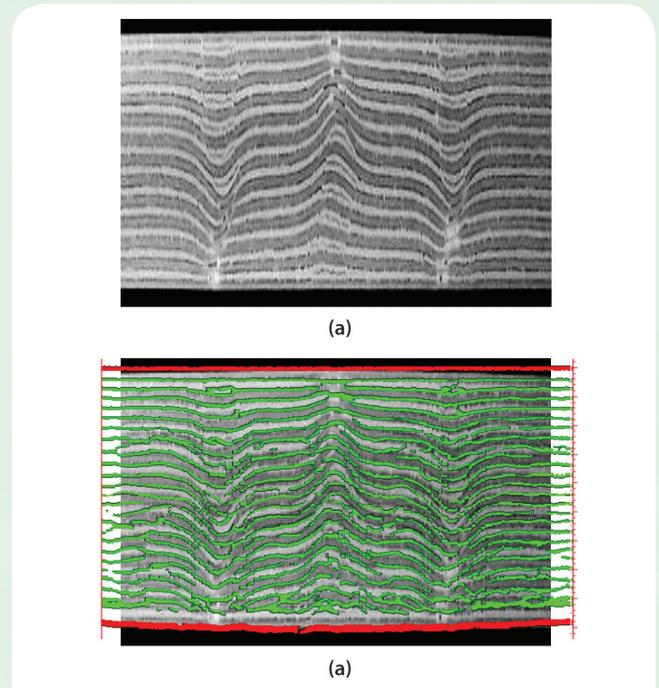
Figure 26. Ultrasonic analytic signal imaging for a specimen containing numerous aligned tape gaps and overlaps, causing out-of-plane wrinkling: the X-ray CT image (a) has an overlay inverted from the analytic signal response (b), where red lines are the front and back surfaces, while the green lines are the resin layers between plies, all determined automatically from the ultrasonic full-waveform data<sup>[2]</sup>
