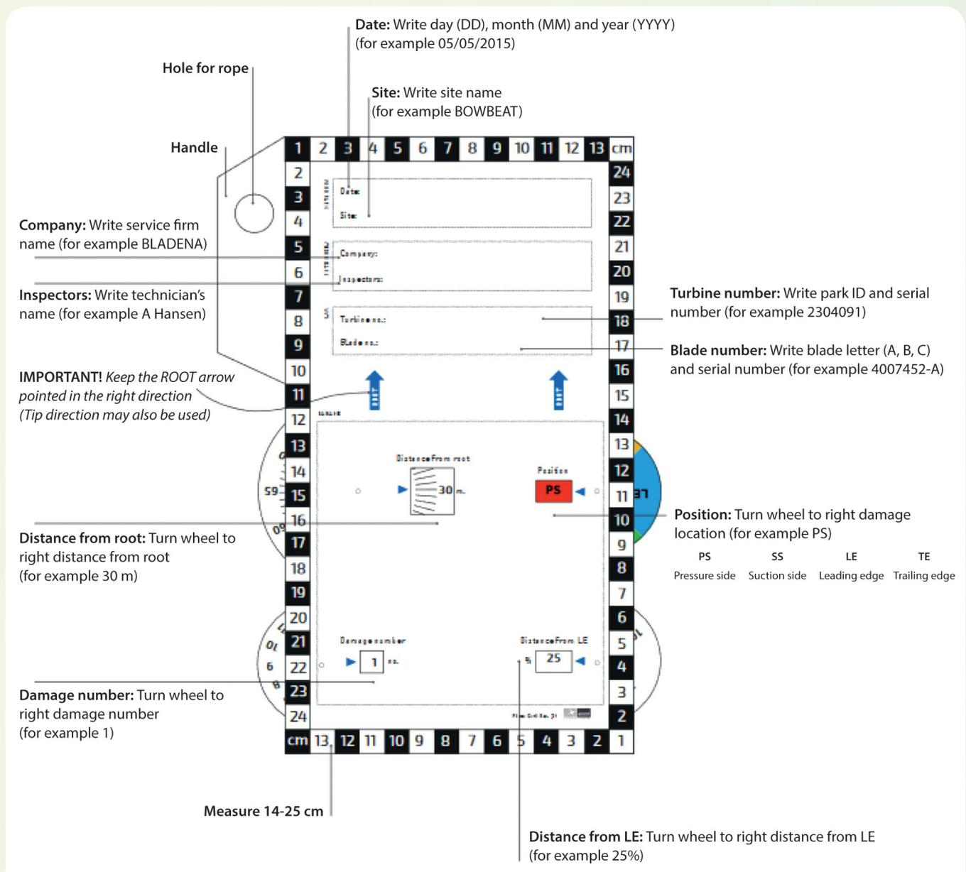
Figure 16. Industry-standard photocard for documenting damage
