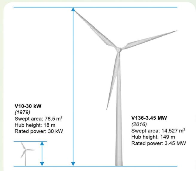
Figure 3. Evolution of wind turbine generators. One Vestas V136 is generating the same amount of power as 115 Vestas V10s
