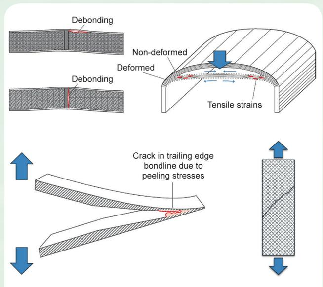
Figure 15. Failure modes: skin debonding and interlaminar failure (top), trailing-edge bondline failure (bottom left) and in-plane strain-based failure (bottom right)
