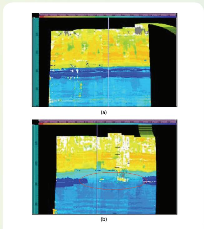
Figure 19. C-scan of internal web-to-blade-skin bonding: (a) well-bonded web (dark blue strip); and (b) disbonded web (circled)
