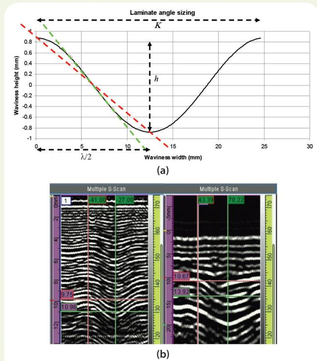
Figure 18. (a) Diagram showing waviness parameters; and (b) waviness imaging of CFRP aerospace laminate at 5 MHz (left) and GFRP wind turbine laminate at 1 MHz (right)
