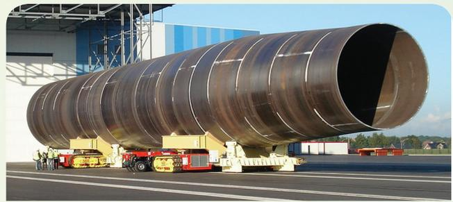
Figure 12. Monopile foundations can be up to 10 m in diameter
