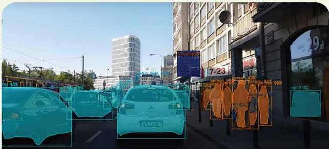
Figure 28. Instance segmentation
