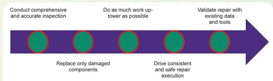
Figure 13. Flowchart demonstrating a good approach to predictive maintenance
