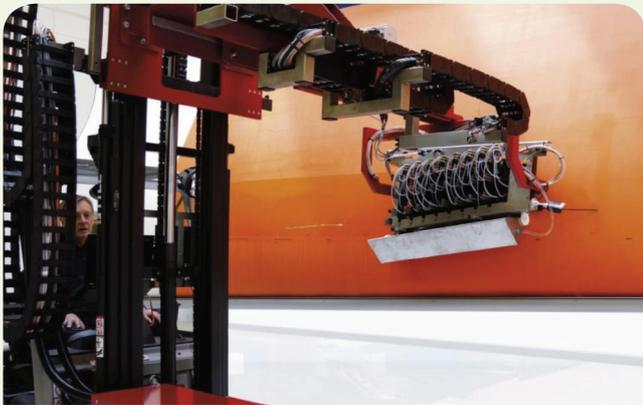
Figure 22. The P-scan system scanning in a manufacturing facility
