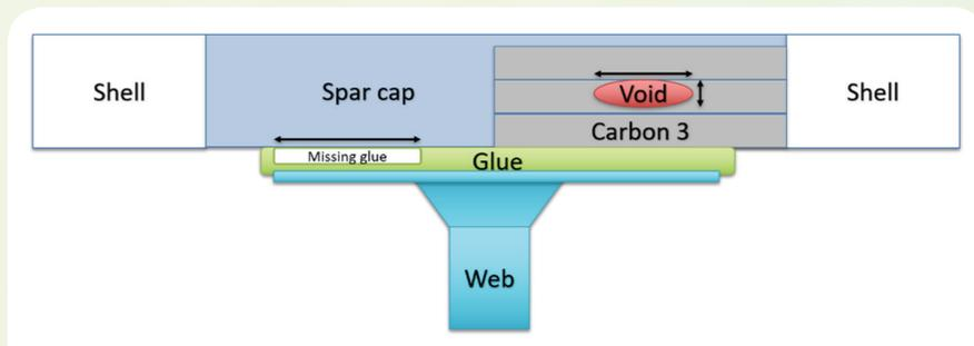
Figure 29. Detecting and measuring defects in the spar cap of a wind turbine blade
