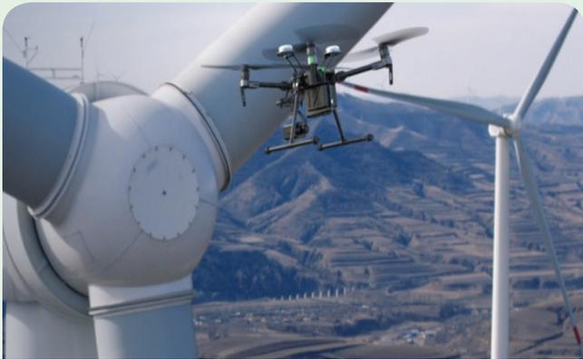
Figure 17. Drone visual inspection
