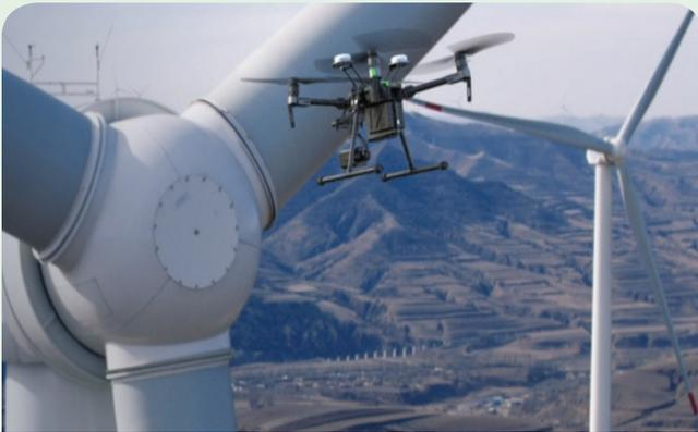
Figure 17. Drone visual inspection
