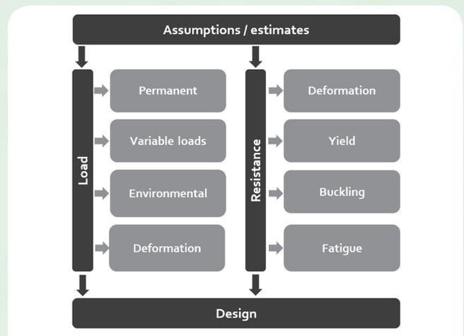
Figure 9. In the early stages of design, assumptions and estimations are made as to the loads experienced by the structure
