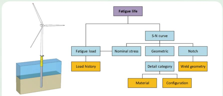
Figure 10. Various parameters affect the fatigue life of the asset
