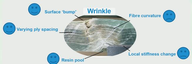
Figure 4. Wrinkle features. A critical parameter is fibre curvature, which is typically difficult to determine non-destructively
