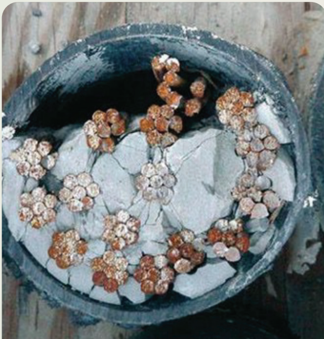
Figure 10. An investigation opportunity is to detect and quantify the voids within post-tensioned cables
