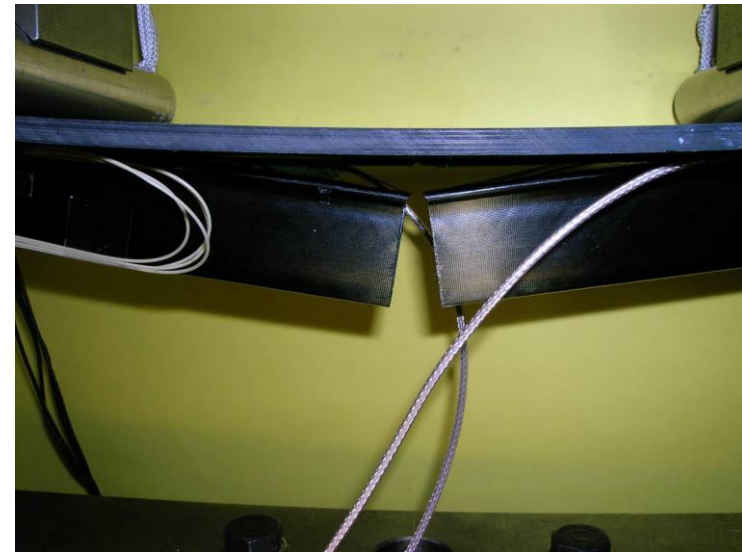
Detection of damaged stiffener disbond and disbond growth under fatigue loading
