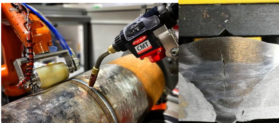
Fully automated robotic welding with integrated NDT for complex multipass welds in high integrity materials
