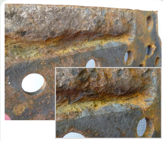
Figure 15. Grooving above the foundation ring on an 80-year-old outer firebox
