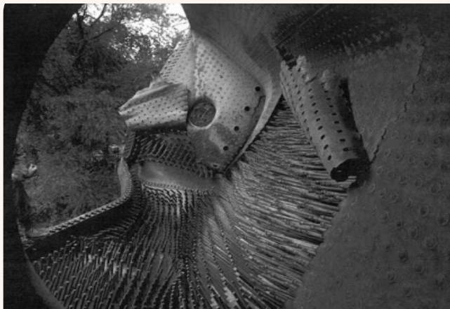
Figure 13. A firebox after a boiler explosion in the USA
