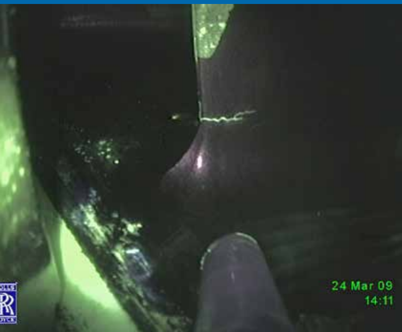
Above: NDT being performed in the 'splash zone' on a North Sea oil rig
