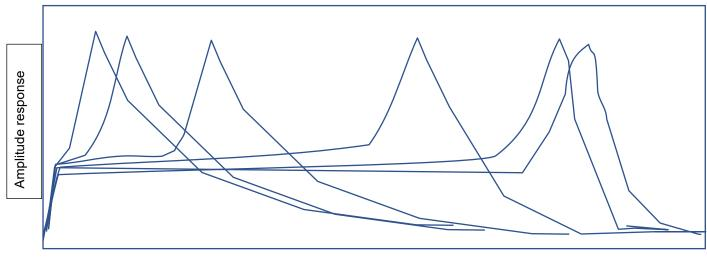
Above the natural frequency, the sensitivity of the measurement drops off rapidly.
