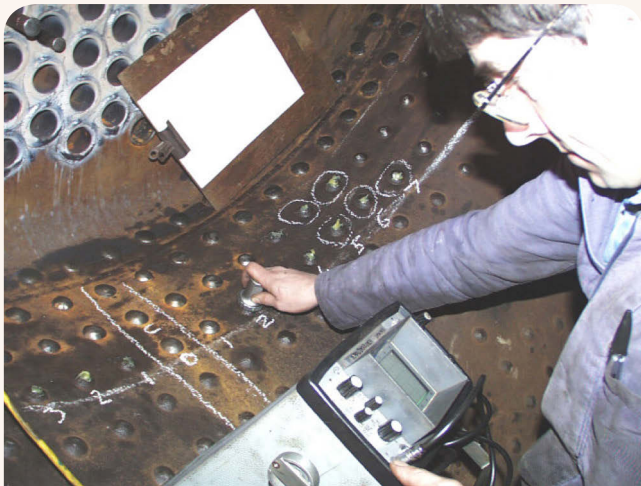
Figure 12. Ultrasonic testing of stays after surface preparation
