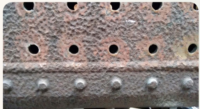
Figure 8. Exterior corrosion making ultrasonic coupling difficult
