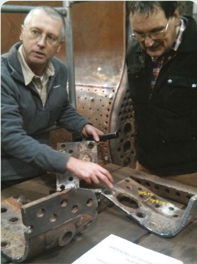
Figure 19. Andy Netherwood (left) explaining the evolution of grooving in the outer firebox
