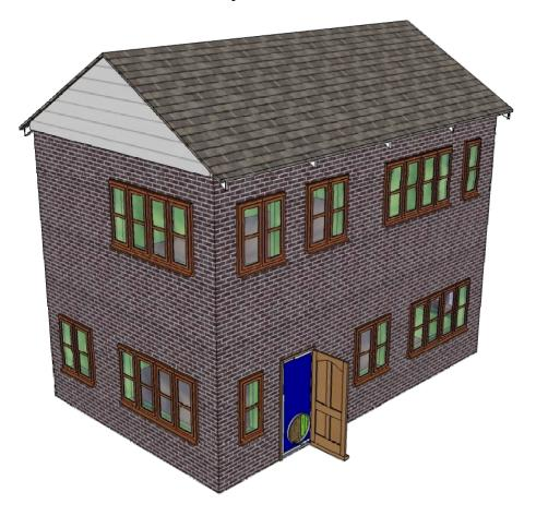
Single fan in single door used for dwellings (door fans typically move 2  $\rm m^3.s^{-1}$ , which allows properties with envelope areas of up to  $720\rm m^2$  to be tested at a specification of 10  $\rm m^3.h^{-1}.m^{-2}$  @ 50 Pa).
