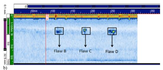
Figure 7 Plane view of the data collected with phased array on the 4mm plate in stainless steel at sensitivity from
