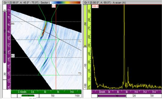
Figure 10 Flaw C phased array data on sample 5mm in stainless steel , sector scan, stand-off 11mm, 3dB, skew 90°
