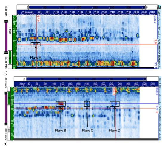
Figure 6 Plane view of the data collected with phased array on the 5mm plate in carbon steel at sensitivity TCG +12dB from
