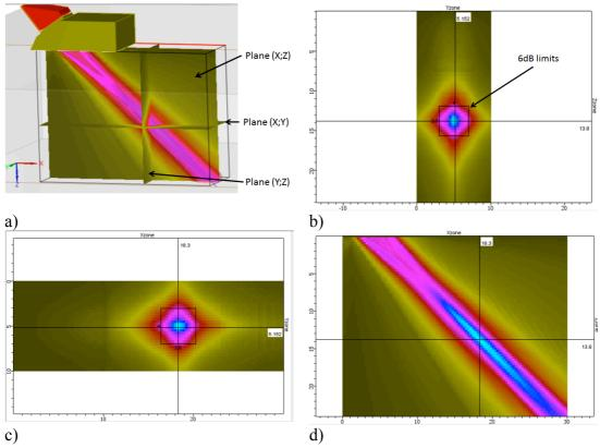
Figure 5 Prediction of the ultrasonic beam profile generated at 45° with the phased array transducer
