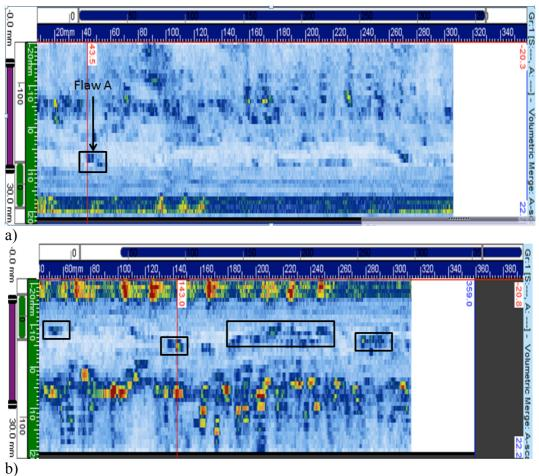
Figure 8 Plane view of the data collected with phased array on the 3mm plate in carbon steel at sensitivity from
