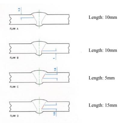
Figure 1 Position of the simulated flaws in the welds
