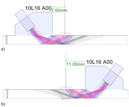
Figure 4 Scan plan for the inspection of the 5mm thick plate (green lines = 70° beam, red lines = 60°, blue line = 45°, pink line = sector scan)
