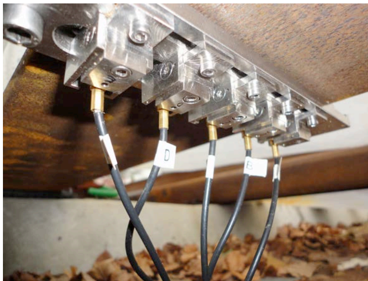
Figure 6. Experimental transducer mounting for rail foot examinations.
