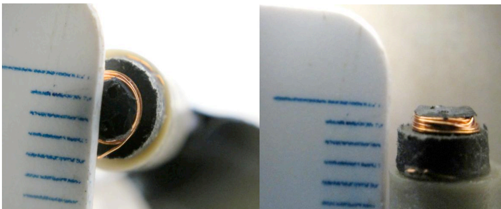
Figure 8. Air-cored probe a) top view b) side view
