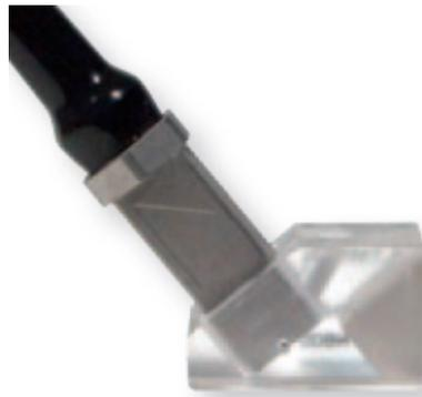
**Figure 3** Picture of phased array transducer 10L16 SA00 N60S manufactured by Olympus and used in the study,
